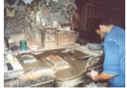
Figure 9: The sand-molding workbench.
