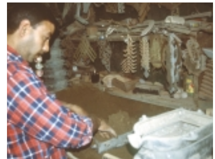
Figure 14: Filling the mold with sand.
