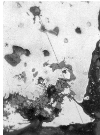
Fig 9: Unetched corrosion (x 1250)
