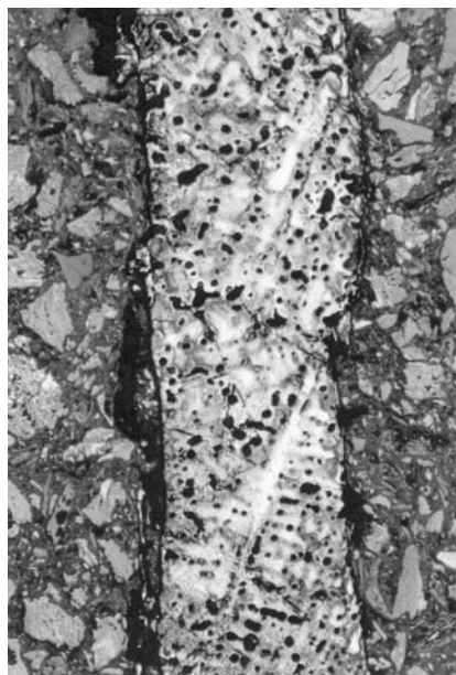
Fig. 2: As-cast dendritic structure (x 250)
